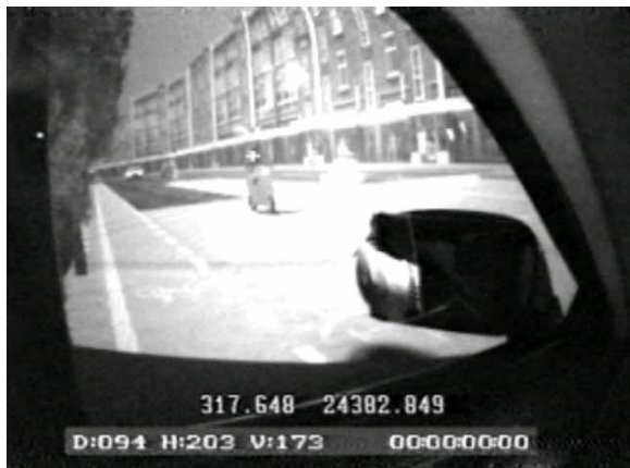
Figure 7. Video image from head-mounted camera, at an instant when eye is fixated on PTW, and head is facing left window of car.
